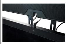
Plug the Audio Cable into the AUDI O jack on the bottom of the screen.
