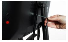
Remove the bottom screws holding the screen to the mount. Place VE SA mount bracket over screw holes and use a bracket screw with wash er to secure. Repeat for other side. Do not tighten.
