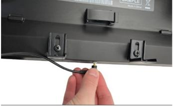
Plug the Audio Cable into the AUDIO jack on the bottom of the screen.
