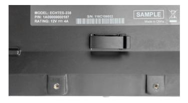
Find the two bracket screw holes on the back of the screen.
