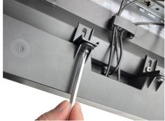
Line up the Soundbar screw holes with the Short bracket screw holes. Use the remainin g 2 screws to secure the Soundbar to the brackets.
