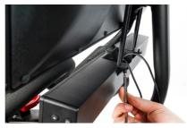
Line up the Soundbar screw holes with the bracket screw holes. Use the remaining 2 screws to secure the Soundbar to the bracket.
