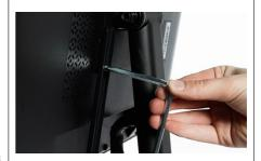
Tighten the bracket screws.
