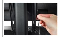
Plug the DC Cable into the DC OU T jack on the back side of the scree n
