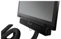
Carefully slide the Soundbar up unti I it is flush with the bottom of the scr een.
