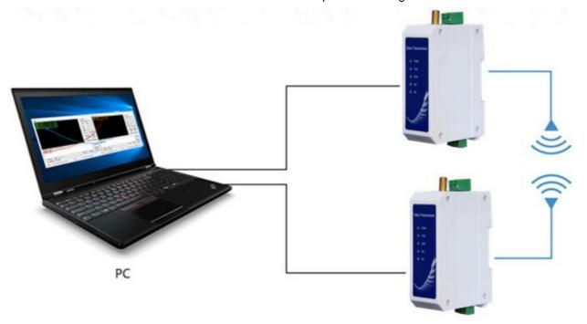
4. Start two serial port debugging assistants, select the serial port baud rate to be 9600bps (default), and the check method to be 8N1 to make serial port transparent transmission.
