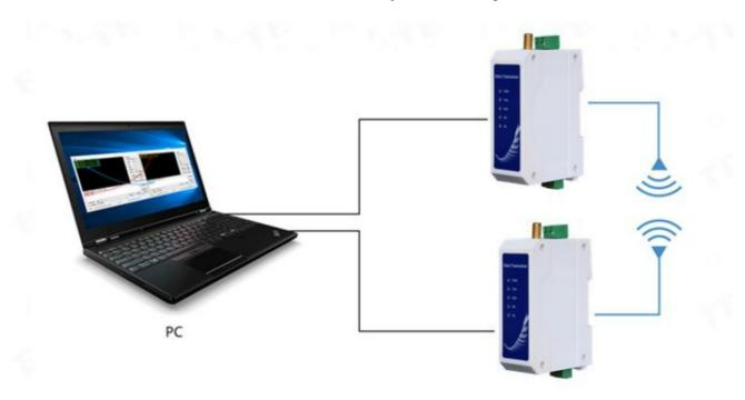
Start two serial port debugging assistants, select the serial port baud rate to be 9600bps (default), and the check method to be 8N1 to make serial port transparent transmission.
