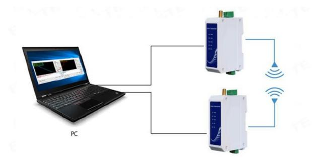
4. Start two serial port debugging assistants, select the serial port baud rate to be 9600bps (default), and the check method to be 8N1 to realize serial port transparent transmission;
