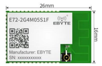
The module leads out all 10 ports of the MCU. Comes with a powerful 48 MHz Arm ® Cortex -M4F processor, an internal integrated power amplifier. powerful peripherals and up to 26 GPlOs, enabling multi-directional development.CC2652RB has the potential to become the best choice of the wireless microcontroller for smart homes, IoT transformation, and industrial automation in the future. Since this module is an SoC module, it needs to be programmed by the user before it can be used.
