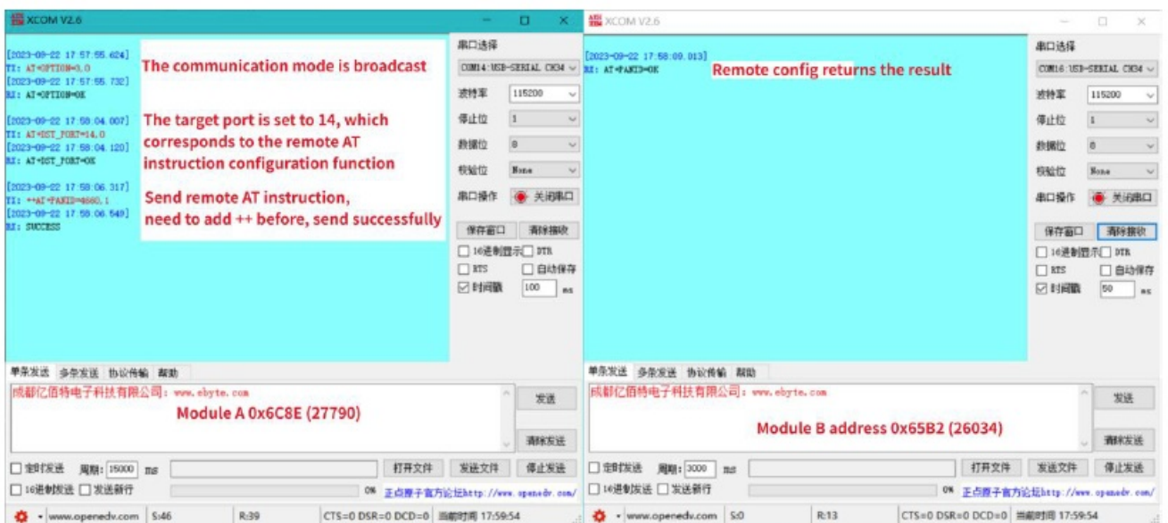
Figure 8.3.1 Remote broadcast configuration steps
