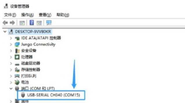
Figure 5.1.2 Device Manager checks COM port
