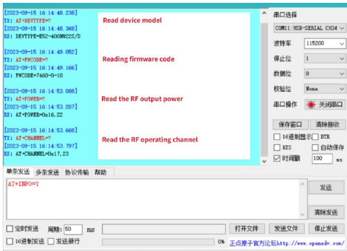
Figure 8.1.2 MCU obtains parameters
