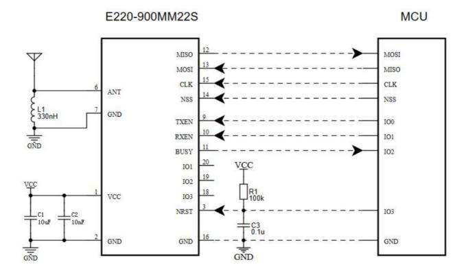
**Note:** The L1 inductor is a protective device used to prevent the device from being damaged due to excessive input power of the antenna. The user should add this inductor when using the module.
