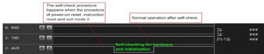
Timing Sequence Diagram of AUX when self-check
