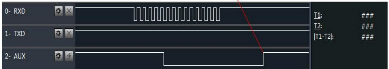
Timing Sequence Diagram of AUX when RXD pin receives Configuration procedure of the module
