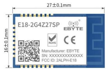
E18-2G4Z27SP adopts the original imported CC2530 radio frequency chip from Texas Instruments (TI). The chip integrates 8051 single-chip MCU and wireless transceiver, and built-in PA+LNA, which greatly expands the communication distance and improves communication stability. And suitable for ZigBee design and 2.4GHz IEEE 802.15.4 protocol.
