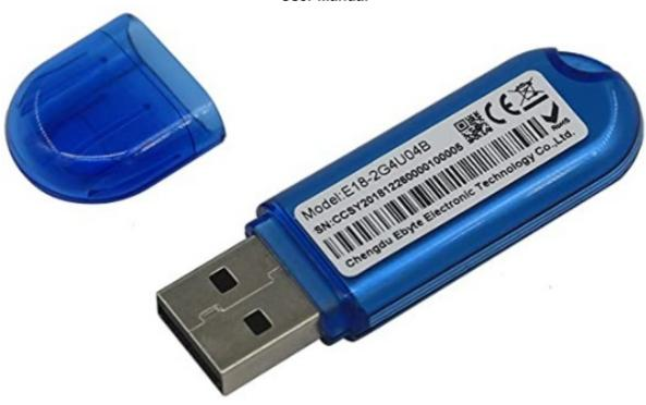
E18-2G4U04B User Manual CC2531 ZigBee USB Wireless packet capture tool
