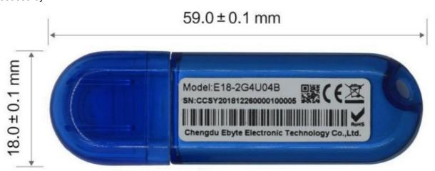
E18-2G4U04B uses the original imported CC2531 RF chip of Texas Instruments (TI) company in the United States. The chip integrates 8051 single-chip microcomputer and wireless transceiver. The factory firmware supports TI Packet Sniffer software to carry out packet capture test. Packet Sniffer can be used to analyze the protocol quickly, and users can also do secondary development.
