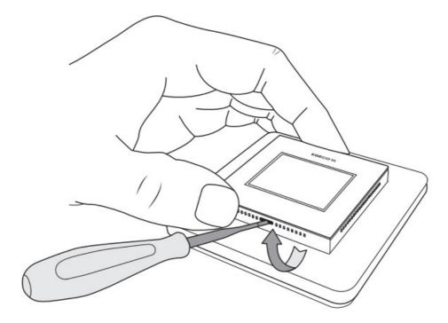
2. Use a screwdriver to gently loosen the front panel.
