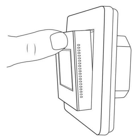
5. Your thermostat will now start automatically. If your thermostat was turned off when the wifi module was installed, you must first press X. Follow the on-screen instructions.
