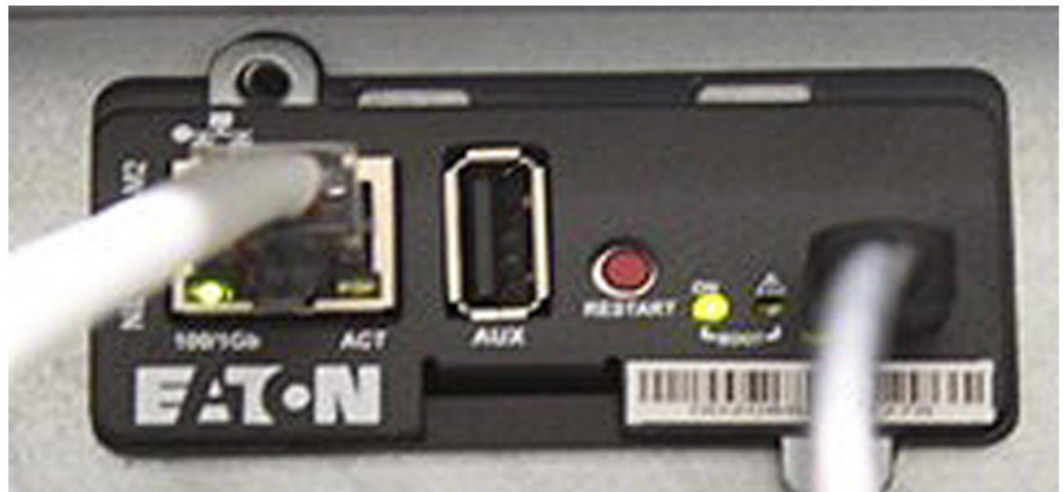
Figure 9. Connect Site Cable to the Network-M2 Card
