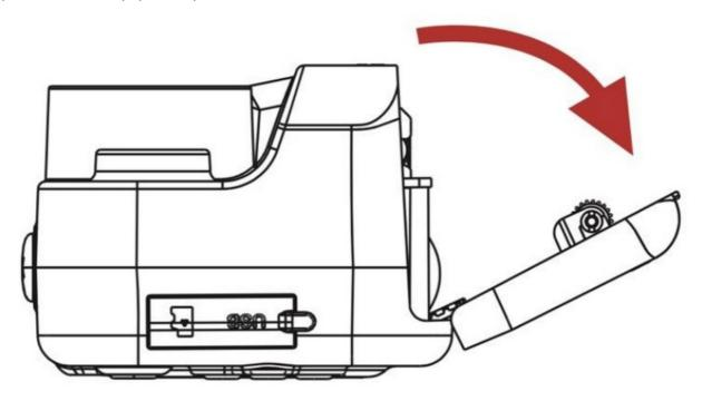
2. Insert the paper roll into the paper tray as shown.
