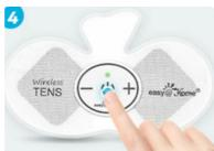
5. To switch modes, hold the "+" button for three seconds. Its beeps correspond to various operating modes. Each time you change modes, release the "+" button and hold it down for another three seconds.
