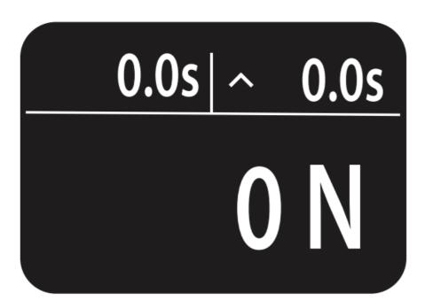
**Step 2** – Start measurement either by pressing the main button again or instruct the patient to start pulling. Measurement will automatically start when the force reaches 5 N for more than 0.5 s.
