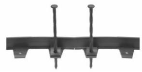
Place the connector on top of the end tabs of each piece. Spike through the holes in the connector and each of the end tabs.
