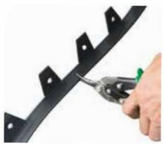
Cut edging at the midpoint between the anchoring tabs using hand snips or a fine tooth saw.
