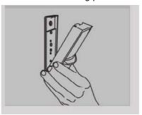
The sensor snaps into the tab at the top.
