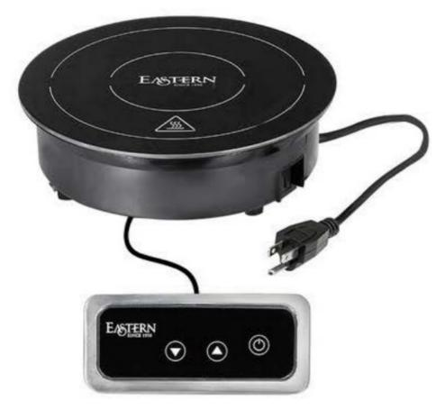
Warming / Holding Induction Range, countertop or drop-in, 9.5/8" round, electric, single burner, 5 position set hold temperature, temperature range:  $145^{\circ}$ -  $190^{\circ}$  F, daisy chain up to 3 units, 120v/60/1-ph, 600 watts, 5 amps, ETL approved.
