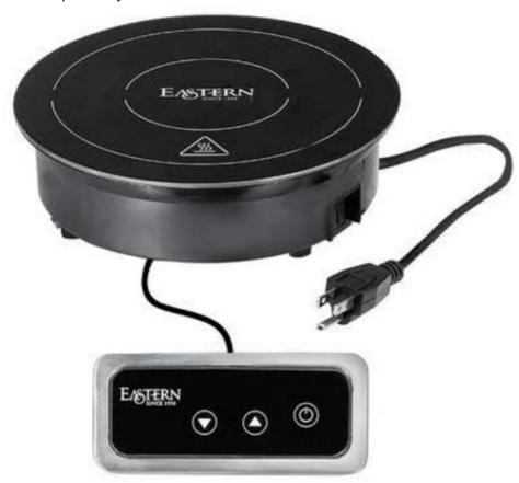
Holding Induction Range, countertop or drop-in, 9.5/8" round, electric, single burner, 5 position set hold temperature, temperature range: 145°- 190 ° F, daisy chain up to 5 units, 120v/60/1-ph, 300 watts, 2.5 amps, ETL approved.
