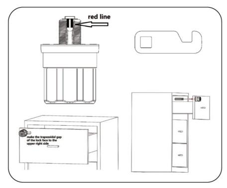
If it is right throw of plate(clockwise turning to lock the cabinet), firstly set the commutator adjuster to (see below black line in the picture), and then make the trapezoidal gap of the lock face to the upper left side, at last fix the lock plate by tightening the screw with a screwdriver.
