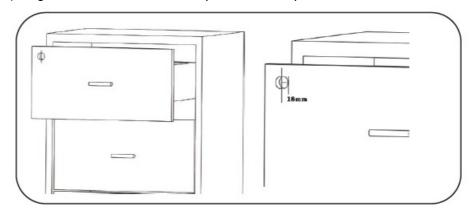
2. Product Installation(1)Lock the Anti-Medlock button .When the keyhole of the lock is vertical to the ground, align the lock with the cabinet keyhole and insert, then fixt it by tightening the screw nut with the wrench.
