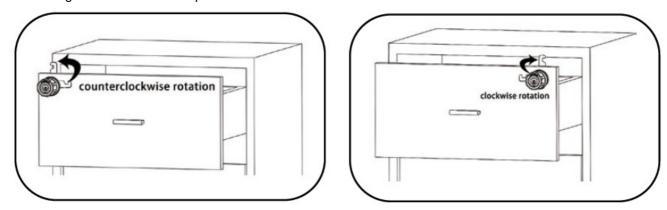
If it is left throw of plate (counterclockwise turning to lock the cabinet), firstly set the commutator adjuster to be(seebelow red line in the picture), and then make the trapezoidal gap of the lock face to the upper right side, at last fix the lock plate by tightening the anti-loose gasket and screw with a screwdriver.
