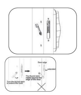
• STEP 6: Fix and install the interior handle on the door. Install (do not over-tighten) the two machine screws through the interior handle and tighten them to the exterior pull. Turn the thumb latch can lock and unlock the door successfully, then tighten the screws.
