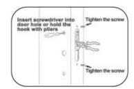
• STEP3: First, ensure that the lock pin goes into the "X" slot in the hub of the thumb latch, then put it through the hub of the mortise lock as shown. Next, turn the thumb latch to test whether you can normally extend or retract the hook. Be sure to test the hook can extend or retract without issue by turning the thumb latch.
