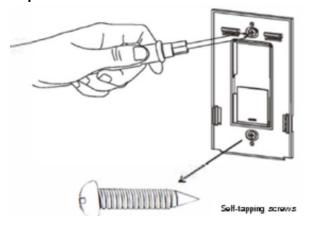
Step 6: Attach the wall plate.
