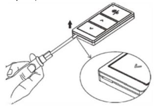
Step 2: Replace the battery (CS2032) with a new one.
