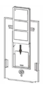
**Step 4:** Attach the bracket with the supplied self-tapping screws.
