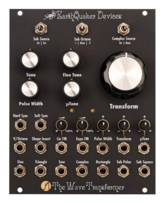
Hey, what's up? Congratulations on your purchase of The Wave Transformer Transfiguration Oscillator. The Wave Transformer is a voltage-controlled oscillator with vintage voicing and over 8 octaves of precise pitch tracking. It has 7 simultaneous wave outputs, including a special Complex output.
