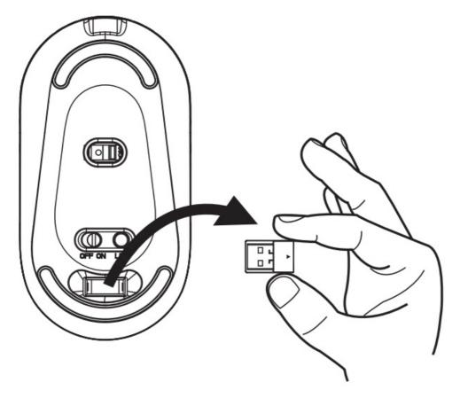
3. Insert the receiver into computer USB Port.
