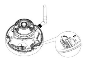
Press and hold the reset button for 10 s to reset the camera
