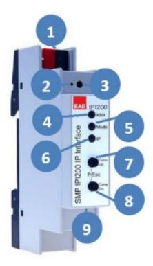
In addition to the normal programming button **9** the device allows activating the programming mode on the device front without opening the switchboard cover. The programming mode can be activated and deactivated via pressing simultaneously both buttons
