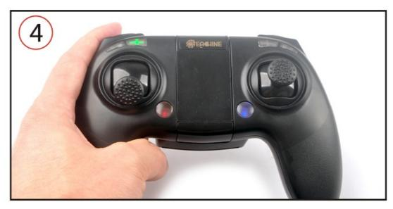
Press AUX1 (CH5) switch to arm the NOVICE-II, you will find "ARMED" notice in the screen of the Goggles. Recommend press AUX2(CH6) to choose Stable mode for the beginner. Happy flight and keep it safe.
