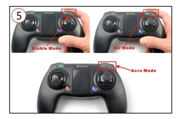
Press AUX2 switch(ch6) to select flight mode (Default is Aero mode)
