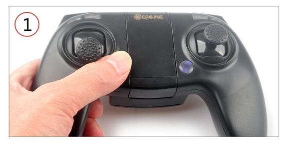
Install 4x AAA 1.5v battery to the radio and Short press the power switch to turn on the radio. If the throttle stick was not at the bottom position the radioter will alarm.
