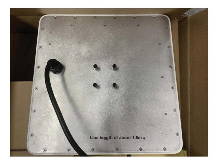
RFID installation instructions: RFID supplies power through red line VCC and black line GND, and communicates through blue line 485a and white line 485b
