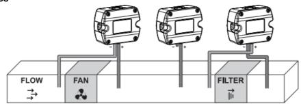
Use a Ø7.5 mm drill for installing the pressure connection nipples into the duct.
