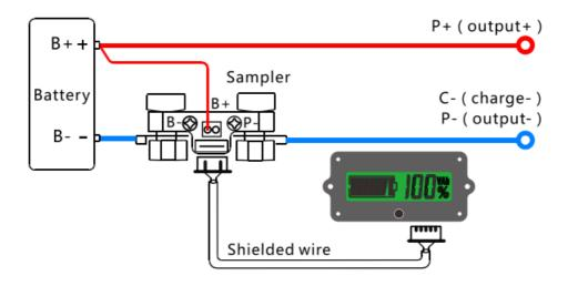
**Attention:** Please connect as shown strictly. The sampler must be connected to the negative circuit, it is forbidden to connect to the positive circuit. If you want to extend the shielded wire, you must use 4 lines of same specification.
