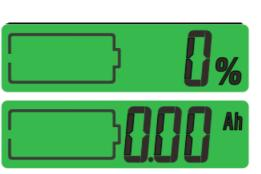
When on first use or change the battery the memory capacity should be set to zero or full: In the main
