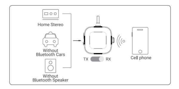
**Receiver Mode(RX)**: Connects to non-Bluetooth receiving devices such as car stereos, wired headphones, and home stereos. This facilitates the wireless transmission of audio from your phone or computer to these devices.
