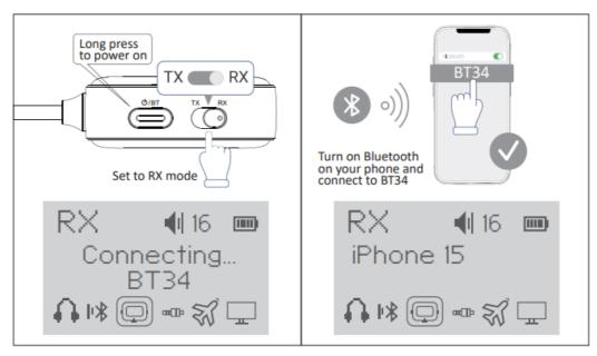
Shift the switch to RX mode and press the "O/st "button for approximately 3 seconds to power on and initiate pairing mode.
