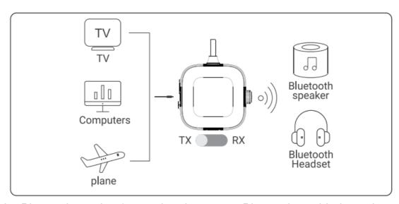
Insert the Bluetooth receiver/transmitter into a non-Bluetooth-enabled speaker device's 3.5mm audio port using a 3.5mm audio cable. Delight in your audio experience.
