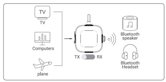
**Transmitter Mode (X)**: Establishes a connection with non-Bluetooth transmitting devices like televisions, airplane entertainment systems, treadmills, and computers. This enables wireless transmission of audio to your Bluetooth headphones or speakers.
