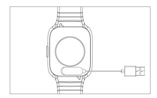
Long press the power key to turn on your watch. If it Doesn't turn on, properly attach the magnetic charging base to the back of the watch, then plug the USB end into a USB port on the computer, charging dock or power bank for charging.
