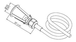
For applications where condensation is likely to happen, certain ways of mounting are required. For probe hanging onto its cable from the ceiling, use the drip water protection HA010503 not included in the scope of supply. This protects the probe and the sensing head against water dripping along the cable. For horizontal mounted probe, a drip water point should be made just before the probe.
