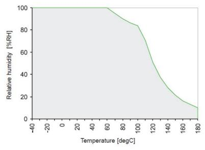
The gray area shows the allowed measurement range for the humidity sensor. Operation beyond this range does
