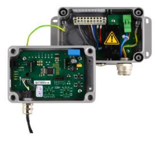
The back cover and the middle active part of the EE23 with metal enclosure must be grounded during operation. The E23 enclosure must be properly closed before power on. Power off the device before opening the enclosure.
