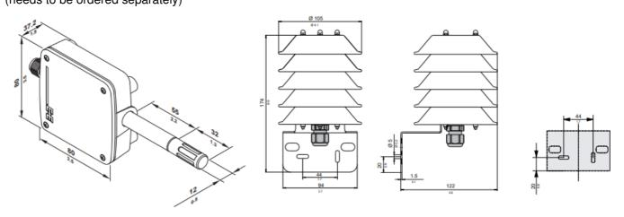
EE210 with cable gland: Use a matching wrench to install the cable gland (in the scope of supply) onto the EE210 enclosure.
