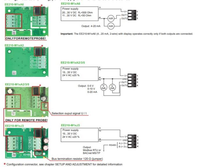
Configuration connector, see chapter SETUP AND ADJUSTMENT for detailed information
