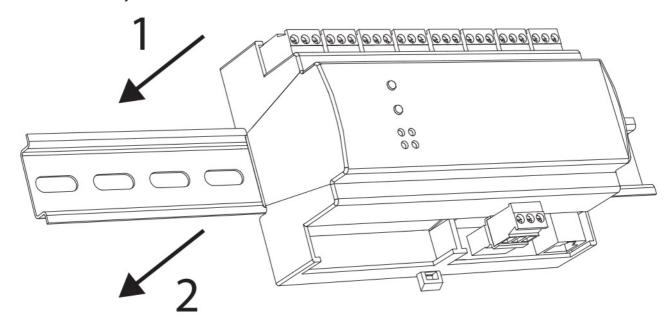
You can also mount the e:cue SYMPL essential 2 Node on any flat vertical surface. Use 3 to 3.5 mm screws for the hanger hole.
