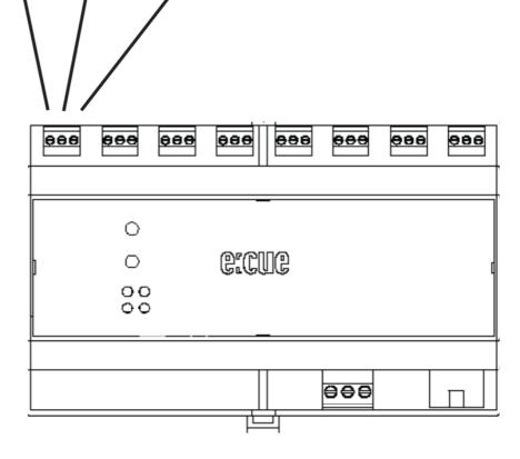
It is recommended to use twisted pair cabling. 120 ohm or 100 ohm 1- or 2-twisted pair shielded cable are suitable for use with EIA-485 (120 ohm) and EIA-422 (100 ohm) devices.
