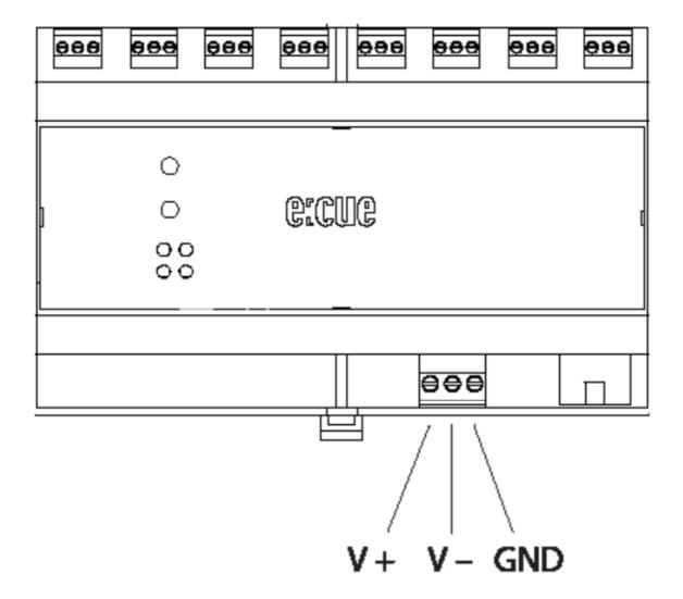
Turn the power on when all cables are connected to the SYMPL essential 2 Node. The device starts operating. The device is in operation when the LED Status is flashing.
