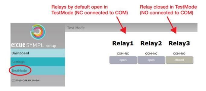
Click the "open" button of a relay to close the relay. Open it again by clicking the button (now "closed") anew. Exit the Test mode by leaving the Test mode page, e.g. go to "Dashboard", or by double-pressing the Identify button.
