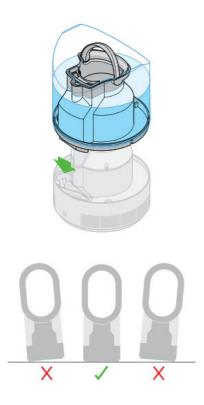
2 Place the tank on top of the base. Ensure the base is on a level surface, otherwise the machine will not operate.
