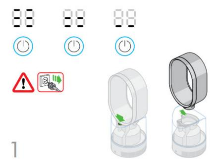
Unplug the machine and push the button to unlock. Lift the loop amplifier away from tank, then tank away from base.
