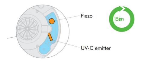
dishwasher. Fill the trough with the recommended acid citric solution until the UV-C emitter and piezo are submerged. Leave for 15 minutes. Drain, rinse and wipe over all surfaces. Repeat if necessary.
