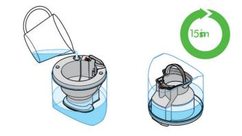
Pour in the recommended citric acid solution. Replace the cap and shake tank for 30 seconds. Then leave to stand. After 15 minutes, empty the tank. Rinse and wipe over all surfaces. Repeat if necessary.
