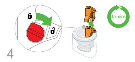
Empty the water tank. To release the water chimney, twist the dial a quarter of a turn. Lift out. Clean thoroughly by immersing in the citric acid solution for 15 minutes. Rinse and wipe over all surfaces. Repeat if necessary. Refit in reverse order, twisting the dial a quarter of a turn to secure.
