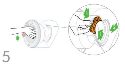
To remove the seal, pinch the securing tabs together and pull out. Clean thoroughly by immersing in the recommended citric acid solution for 15 minutes. Rinse and wipe over all surfaces. Repeat if necessary. To refit, push back in so the tabs click and the fit is secure.
