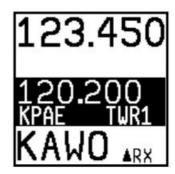
**Note:** the arrow on the top bar that points to the active frequency, and the up arrow on the RX area of the control panel display that points "up" to the active frequency:
