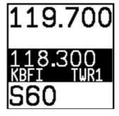
Use the TWR, ATIS, GND, and ATC buttons on the control panel to send the associated airport frequencies to the standby frequency location:
