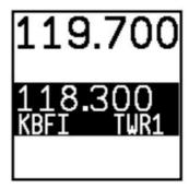
• With a valid Com frequency highlighted, (a 25kHz frequency on the SV-COM-X25 and SV-COM-C25 and an 8.33kHz on the SV-COM-X83) press the TUNE COM button to send the frequency to the standby frequency:
