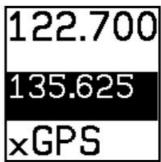
Without GPS position, airport loading, and TWR/ATIS/GND/ATC will not be available. You may see this annunciation as SkyView starts up or when the aircraft does not have GPS reception (for example, when inside the hangar).
