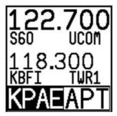
Press the dual concentric knob on the control panel to load the airport to the control panel (or press APT to cancel your selection):
