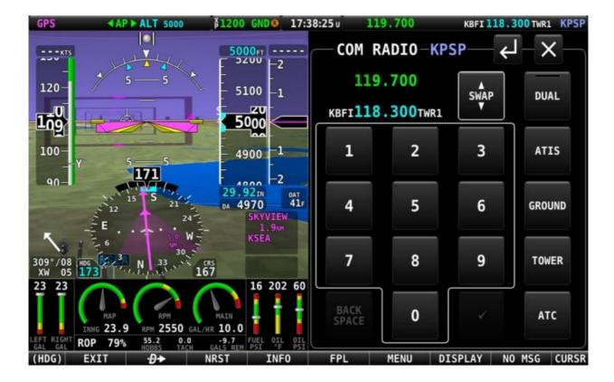
The on-screen COM RADIO control panel offers all the same function controls as the external control module except:
