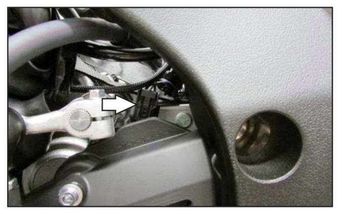
Make sure to connect to the LOWER set of injectors.
