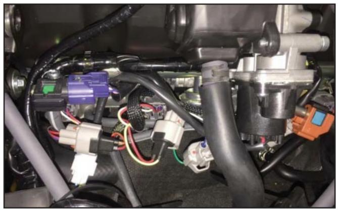
10. Unplug the crank position sensor connector.
