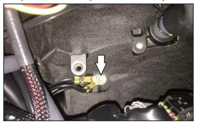
8. Plug the PC6 in-line of the stock gear position sensor and wiring harness. This connection is located on the left side of the engine above the sprocket cover.
