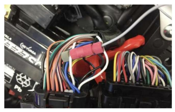
7. Attach the ground wire of the PC6 to the common ground location towards the rear of the engine.
