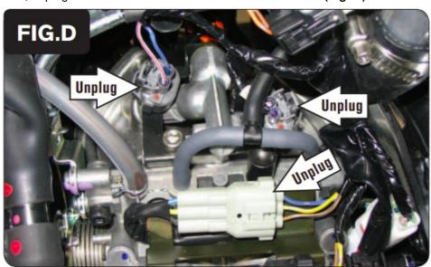
The TPS connectors are the pair of GREY 3-pin connectors.
