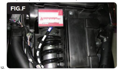
13. 12v source for Auto-tune – RED wire of the 6-pin tail light connecto
