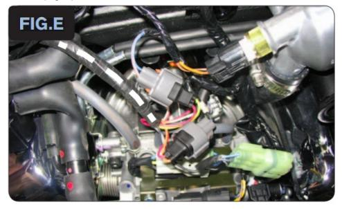
The pair of PCV leads with ORANGE colored wires go in-line of the front cylinder fuel injector and stock connector. Likewise, the pair of PCV leads with YELLOW colored wires go in-line of the rear cylinder fuel injector and stock connector. 10 Plug the pair of PCV leads with 3-pin connectors in-line of the stock TPS connectors. **FIG.E**
