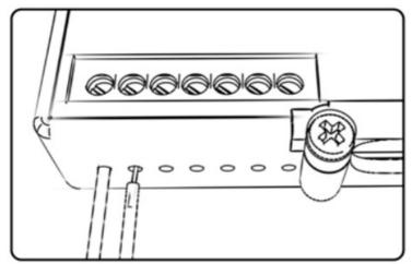
To input wires into the PCV first remove the rubber plug on the backside of the unit and loosen the screw for the corresponding input. Using a 22-24 gauge wire strip about 10mm from its end. Push the wire into the hole of the PCV until is stops and then tighten the screw. Make sure to reinstall the rubber plug.
