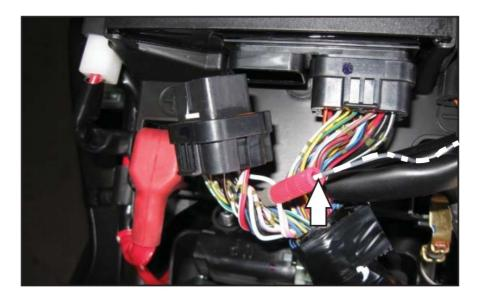
8. Attach the ground wire of the PC6 to the negative side of the battery.
