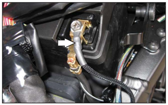
9. Using the supplied Velcro, secure the PC6 to the plastic cover under the right hand side cover. Mount the PC6 behind the stock electronics.
