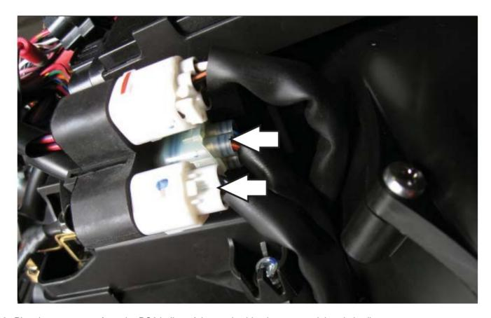
6. Plug the connectors from the PC6 in-line of the stock wiring harness and throttle bodies
