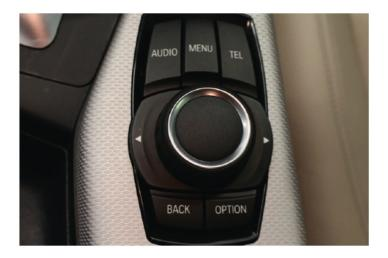
Press and hold "BACK" button for 2 seconds to switch between original NBT and Dynavin menu
