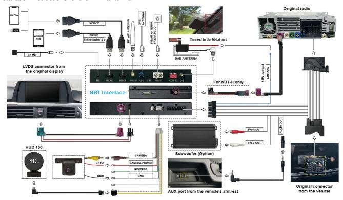
For a quick system start, connect the yellow power wire to the car battery as shown below:
