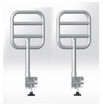
2. Clamp the rail bracket over the edge of the bed deck with the vertical sliding steel plate positioned on the inside of the bed frame. Tighten the two Allen screws and rotate the turn knob underneath the bracket clockwise until the rail is secured in place. Repeat the procedure to install the bed rail on the other side.
