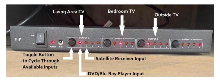
\*In this example – The Living Room TV (Output A) is connected to the DVD Player (Input #1); the Bedroom TV (Output B) is connected to the Satellite Receiver (Input #2); and, the Outside TV (Output C) is connected to the DVD Player (Input #1).
