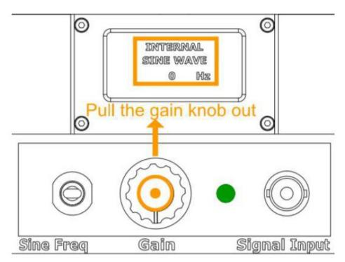
Raise or lower the Sine Frequency Generator Switch to the desired Sine frequency. Adjust the Gain of the amplifier by turning the Gain Knob clockwise. The frequency of the generated sine signal will be visible on the LCD Screen.
