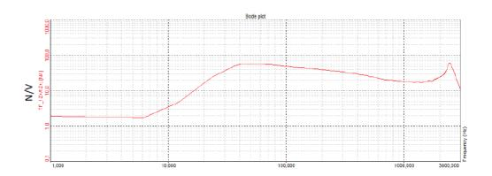
FOR FIXED FREQUENCY SINE TESTING, APPLICATION OF VOLTAGE LEVELS ABOVE 1V FOR LONG DURATIONS (>1MIN) CAN PERMANENTLY DAMAGE THE SHAKER.
