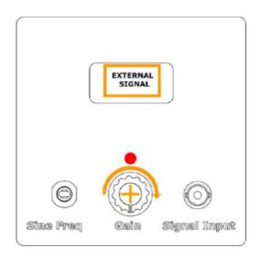
**3.1.2-) Internal Signal Mode:** The amplifier can generate sine signal from 1Hz to 15kHz with 1 Hz increments that the user can adjust with the Sine Frequency Generator Switch. Connect DC power source and drive signal to shaker power input. Pull the Gain Knob out.
