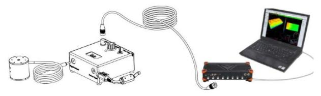
The Gain Knob is a push-pull and rotational switch. The amplifier is in External Signal Mode when the Gain Knob is pushed in and the amplifier is in Internal Signal Mode when it is pulled out.
