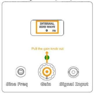
Raise or lower the Sine Frequency Generator Switch to the desired Sine frequency. Adjust the Gain of the amplifier by turning the Gain Knob clockwise. The frequency of the generated sine signal will be visible on the LCD Screen.
