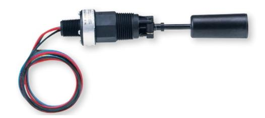
The Model L8 Flotect® Liquid Level Switches are float switches constructed of polyphenylene sulfide, Ceramic 8 and 316 SS. This liquid level switch provides accurate set point control of liquids with specific gravities as low as 0.6.
