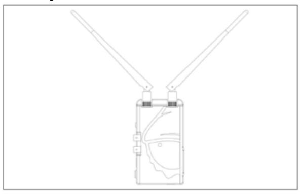
Position the antennas on the transmitter and receiver as shown in the illustration. This ensures the best possible RF performance.
