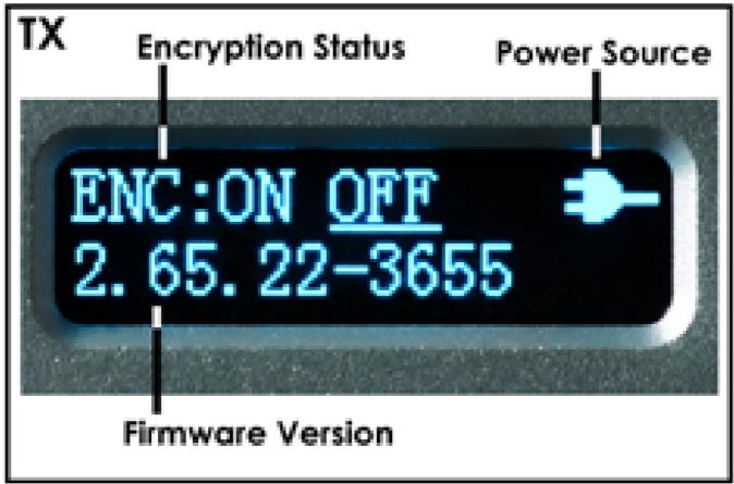
**IMPORTANT**: Switching back and forth between two encrypted systems is not possible. You cannot slip into an encrypted wireless system if your receiver was not initially linked to the transmitter. If you want to add a new receiver to an encrypted system, you need to link the whole system again.
