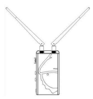
Position the antennas on the transmitter and receiver at right angles as shown in the illustration. This ensures the best possible RF performance.
